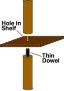
Once all the shelves are of a satisfactory shape, mark the positions of the four holes on the top shelf. The diameter of these holes should be somewhere around 3/8 inches. The precise diameter of the holes should be matched to whatever thin dowel you have available (see next section for an explanation of why you need these).
